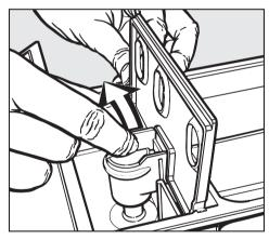
■ Remove the siphon tube from compartment <a href="#">№1</a>.
